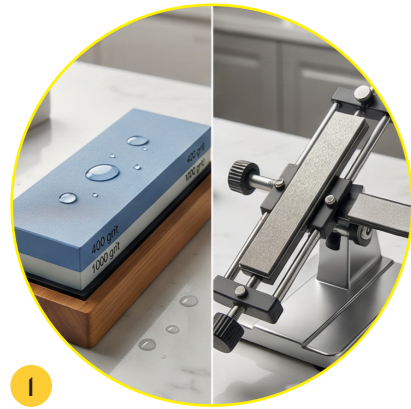
1 Use a whetstone (recommended) or a quality guided sharpening system.
